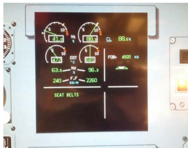
Figure 1. Indications of the Auto Throttle in idle showing four of the five cues: (1) a discrepancy between the N1 axis speed indications of the left and right engines; (2) deviations of the exhaust gas temperature (EGT); (3) rotation speed of the secondary axis N2; (4) deviation in fuel flow (FF) between the two engines.
