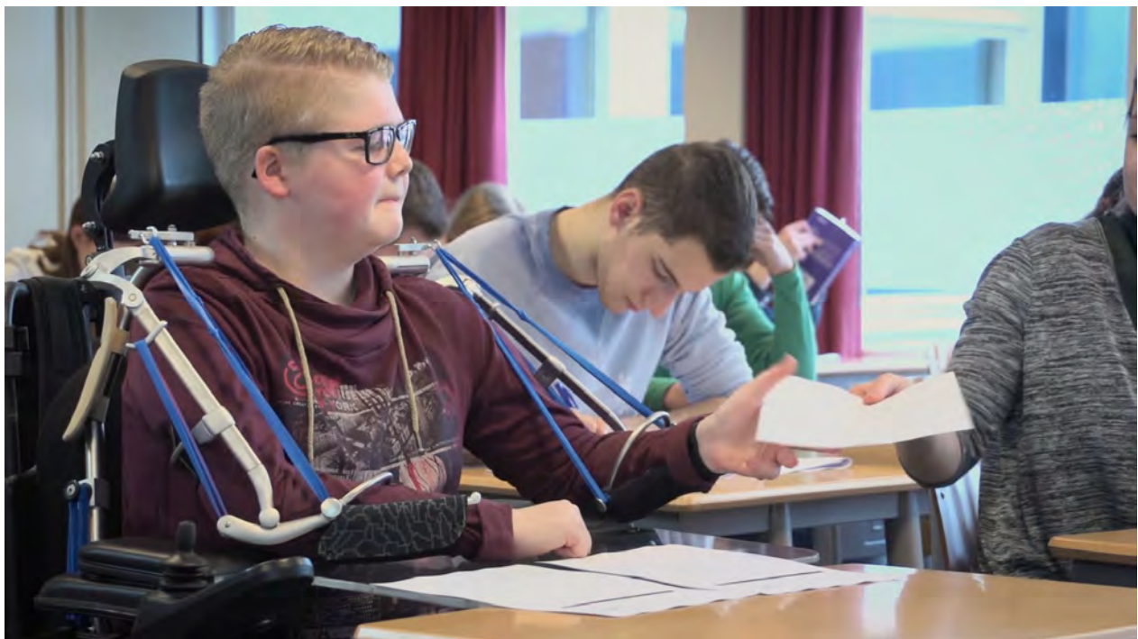
Figure 1. The A-gear (Flextension), first prototype of a passive exoskeleton for Duchenne boys, which is being developed further by Yumen Bionics
