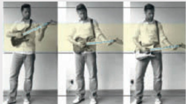
Figure 2. User standing with the guitar in three different positions according to strap length; the tendency to neck dive increases as the strap length increases
