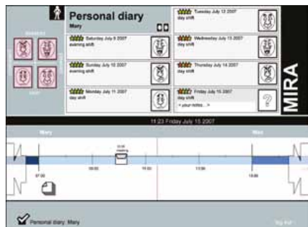
Figure 4. Screenshot of the prototype in human mode (translated from Dutch), illustrating the function 'perception of the shift'. The nurse can indicate how (s)he perceives the shift by choosing a face (upper part left) corresponding with her (his) mood: pleasantly calm, pleasantly stressed, unpleasantly calm or unpleasantly stressed (based on Desmet, 2002)
