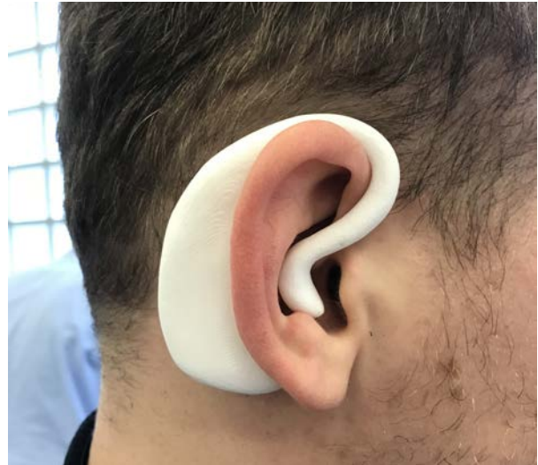
Figure 3. Potential user wearing and testing the comfort level of the 3D-printed average model.
