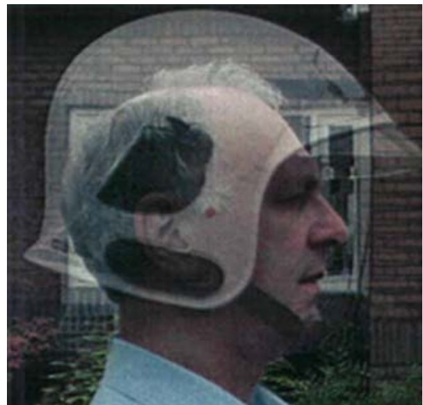
Figure 9. Superimposed images of a photo of a head and head/helmet combination to provide insight in fit.
