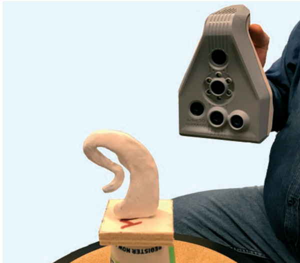
Figure 2. Scanning of the handmade polymorph ear models using Artec Space Spider.
