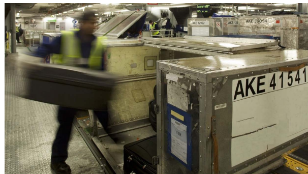
Figure 1. Loading a ULD with partially closed topside; to the left of the handler, bags arrive on a conveyor belt. This situation is called a build lateral, for 'building' a flight.
