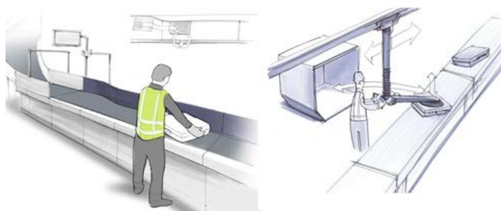
Figure 2. Sketches for brainstorm session (left: reduce reach; right: lifting aid).
